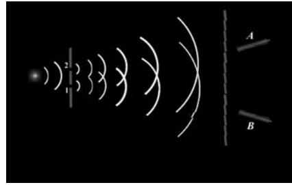
Figure 2. Modified two-slit experiment in which a venetian blind replaces the image screen and a pair of telescopes could be used, if the blind is opened, to determine which slit each photon traverses. (Credit: Author)
